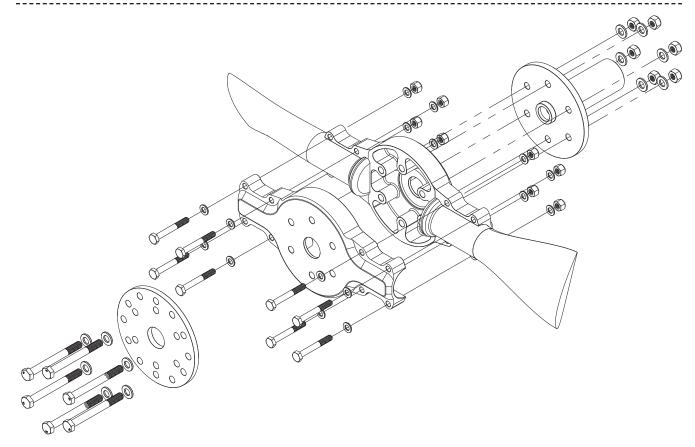
Assemble the propeller as shown in the diagram above.
