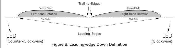
The leading-edge down (LED) direction can be either clockwise (CW) or counter-clockwise (CCW) depending on whether you have a left-hand-rotation or right-hand-rotation propeller.
