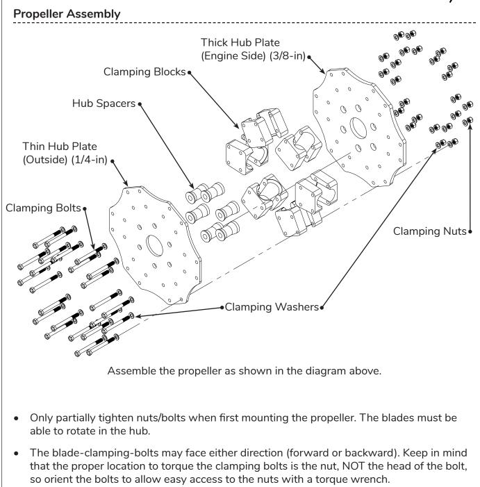
• The six propeller-mounting-bolts will either have drilled-heads to facilitate safety wire OR they will be secured with a Nyloc nut. The proper method of installing bolt safety-wire is beyond the scope of this manual.
