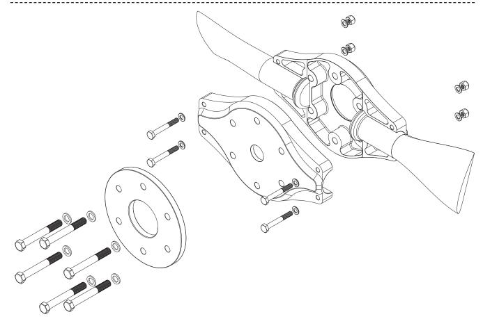
Assemble the propeller as shown in the diagram above.
