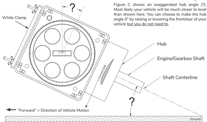
Figure C: Hub Angle Measurement
