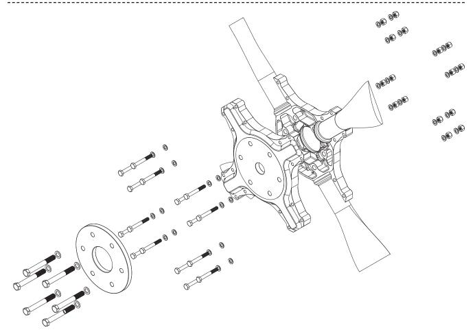
Assemble the propeller as shown in the diagram above.
