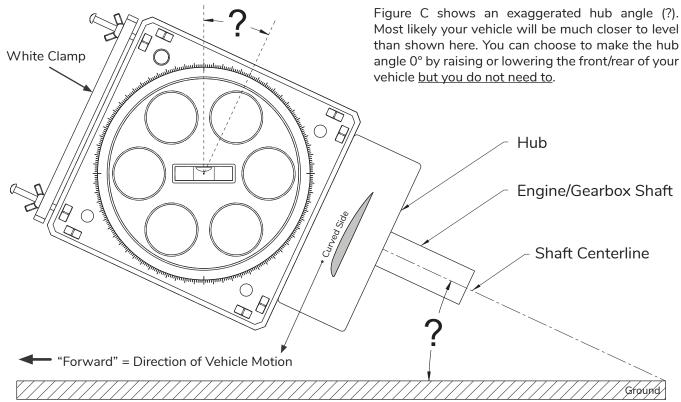
Figure C: Hub Angle Measurement
